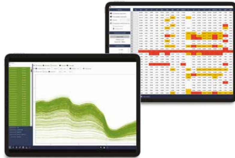
It is a software that is used to import spectra saved in SP3 (or CSV) format and to process them. In its free version, it is used to query SP3 files and to convert them into CSV format to be used with common spreadsheets.
